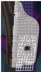
Using contact to mimic the real state. As the contact is non-linear, using intermittent eigenvalue method to solve the vibration behavior in LS-DYNA.
