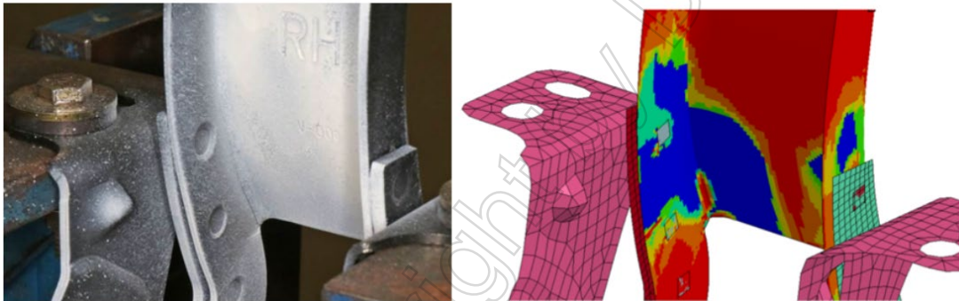
Fig.6 Test vs. Fatigue Life prediction – Simplified Model
