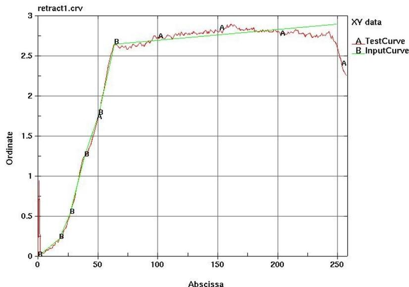
Fig. 5 Approximating a test curve by a series of straight line
