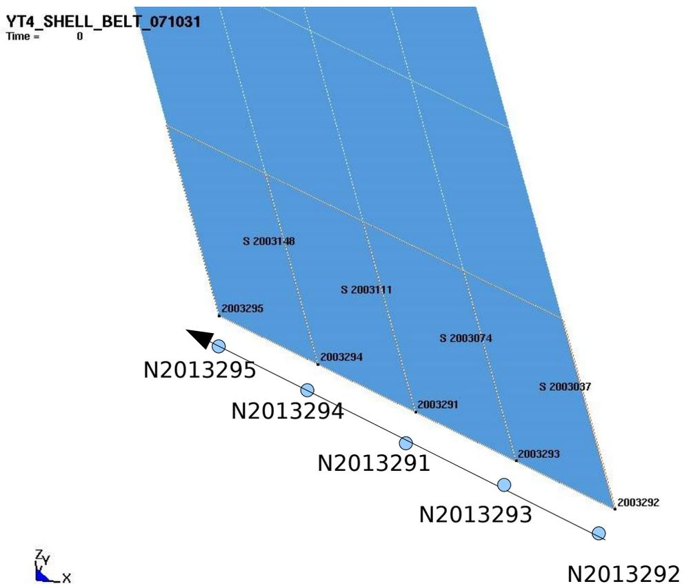
Fig. 4 Edge-node set and retractor node set, -SBRNID
