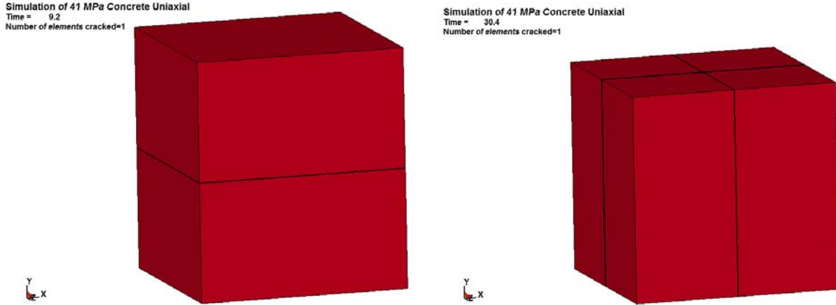
Figure 20 Single tensile crack plane introduced in unit cube when the uniaxial tensile strength is reached (left) and double orthogonal tensile crack planes when compressive strength is reached.
