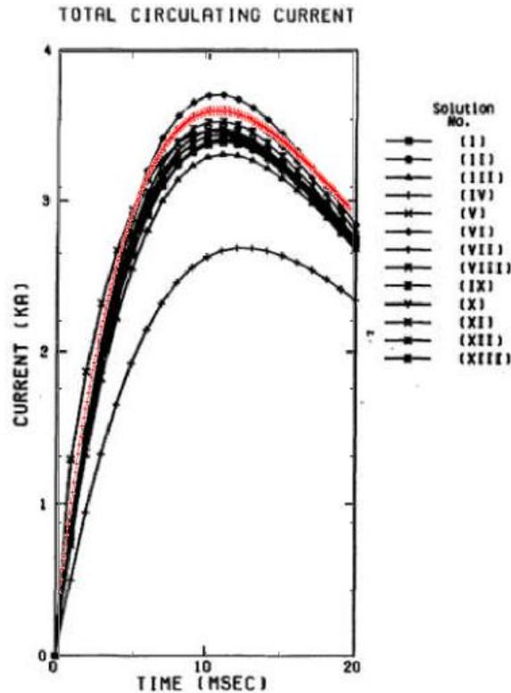
Figure 3 Comparison of the time variation of the circulating current in the FELIX brick between the reference results given by different codes (in black & white) and the LS-DYNA simulation (in red).
