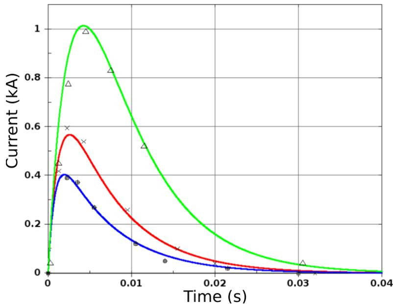
Figure 6 Preliminary comparison for the induce current between LS-DYNA results (full line) and experimental points. From top to bottom: Copper (in Green), Aluminum (in Red), and Brass (in Blue)
