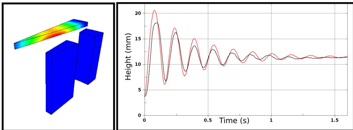
Figure 15 Lorentz Force fringes and Comparison between the experimental results (in Black) and the LS-DYNA numerical results (in Red).
