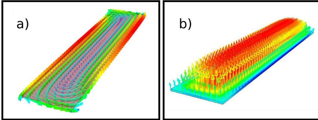
Figure 5 a) Current density vectors, b) Magnetic field vectors
