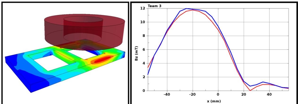
Figure 11 Current Density Fringes and  $B_z$  magnitude variation along the A-B line. Comparison between LS-DYNA (in Red) and reference experimental (in Blue) results.
