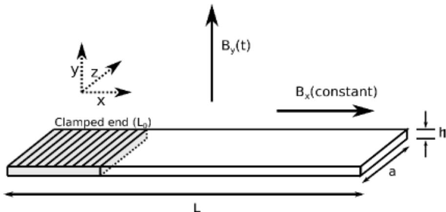
Figure 4 TEAM 12 sketch: L=487 mm, a=100 mm, h=3.175 mm, L<sub>0</sub>=76 mm
