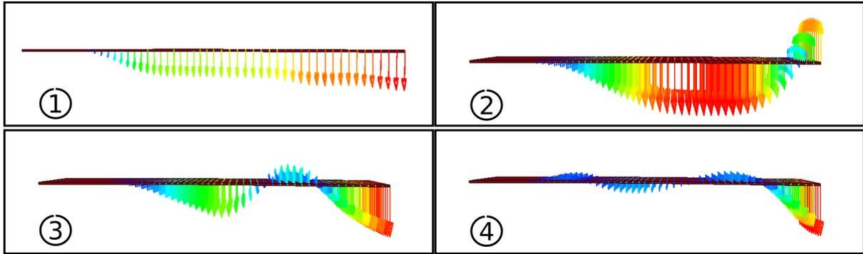
Figure 7 Characteristic Four Modes of Vibration. Acceleration Vectors
