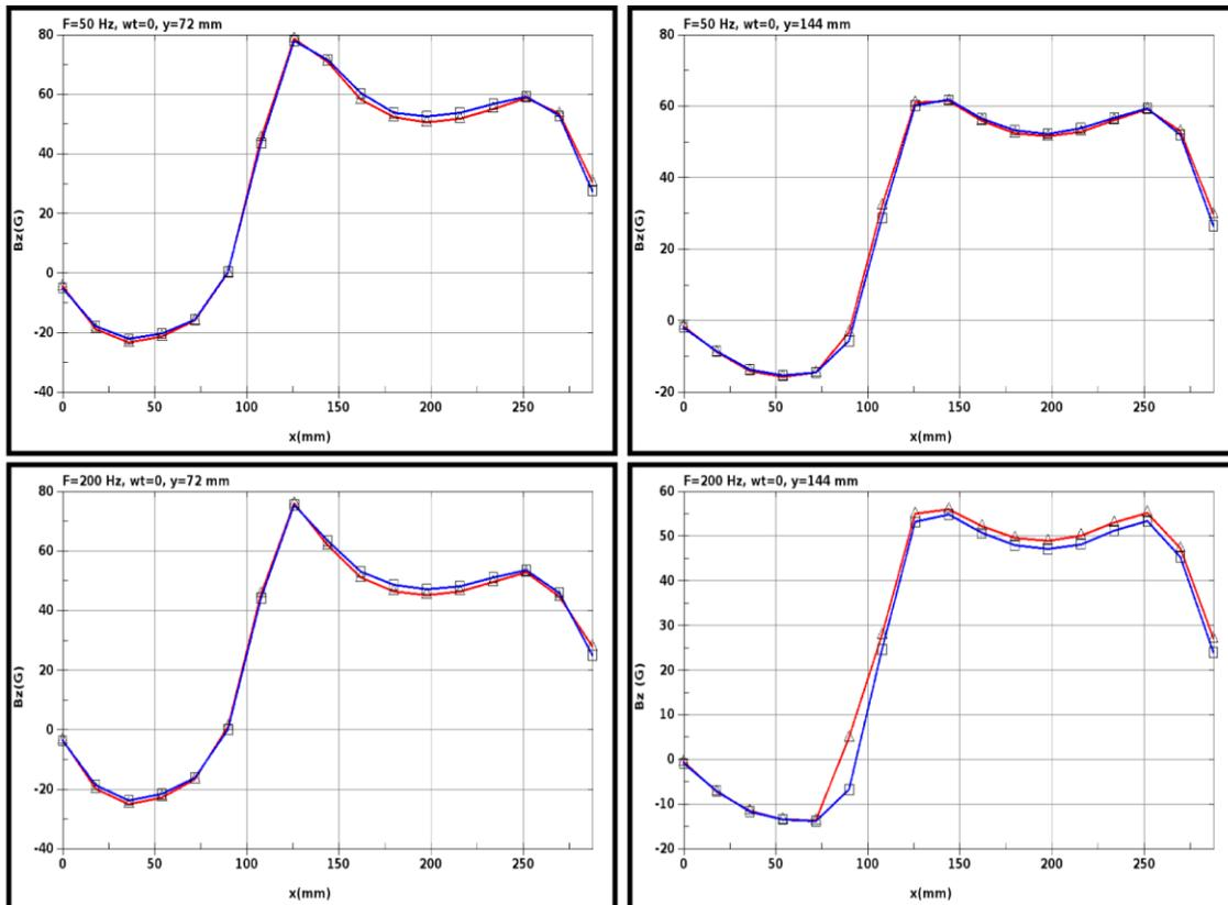
Figure 13  $B_z$  ( $G=10e-4$  T) variation along the A1-B1 ( $y=72$ mm) and A2-B2 ( $y=144$  mm) line at time  $wt=0$ . Comparison between LS-DYNA (in Red) and reference experimental (in Blue) results.
