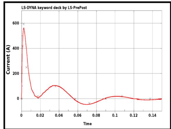
Figure 8 Current and Deflection at the free end (in Red) and 167 mm from the free end (in Blue). Comparison between LS-DYNA results (full line) and experimental results (points).
