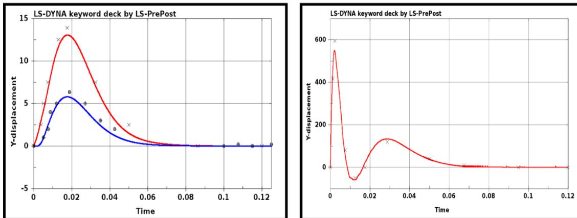
Figure 9 Current and Deflection at the free end (in Red) and 167 mm from the free end (in Blue). Comparison between LS-DYNA results (full line) and experimental results (points).
