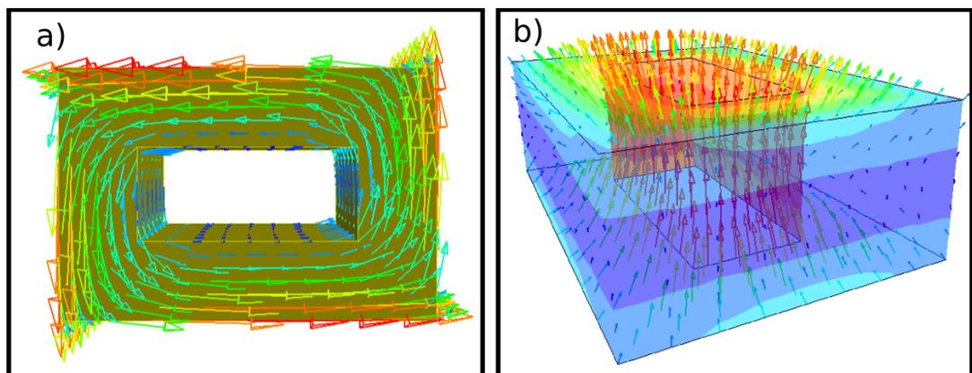
Figure 2 a) Current density vectors, b) Magnetic field vectors
