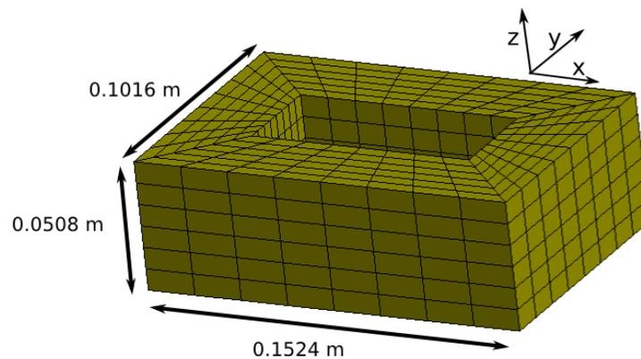
Figure 1 TEAM 4 Geometry and Mesh. Central hole:  $0.0889 \text{ m} \times 0.0381 \text{ m}$
