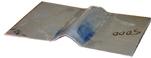
Figure 10: Electromagnetically formed experimental part
