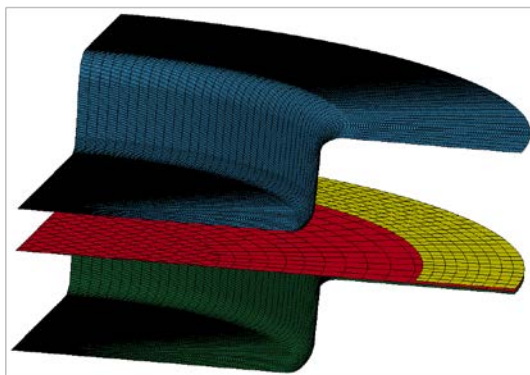
Figure 18-65: Quarter segment of FE model: tools and blank
