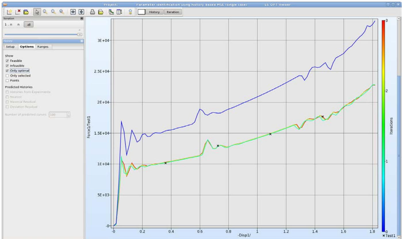
Figure 17-3: Target and computed curves, only optimal curves are displayed for all iterations
