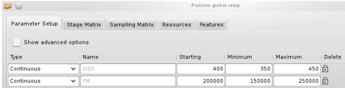
Figure 5-10: Outer level global setup. SIGY and YM are automatically detected in the input file (i.e. inner level .lsopt file) and locked as they are Transfer Variables in the inner level.
