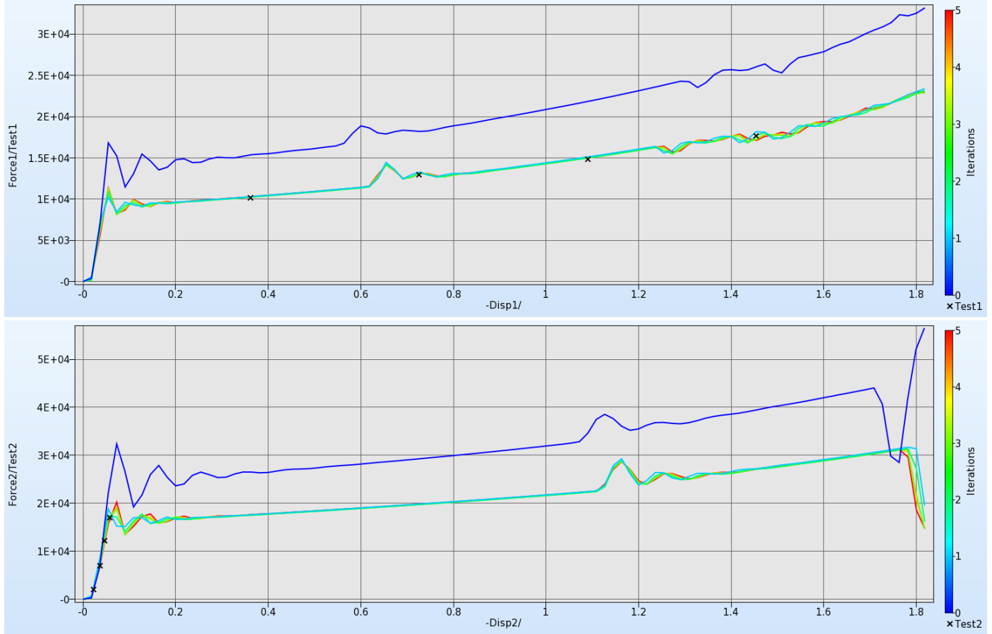
Figure 19-12: Comparison of optimal force-displacement curves and test data. The simulation curves are colored by iteration
