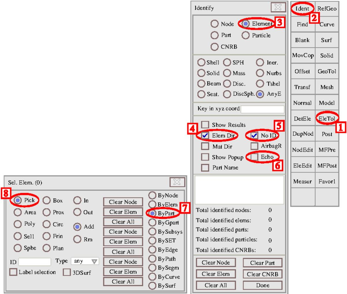
Figure [0-6]. Checking element directions (N1-N2) by part using LS-PrePost4.0.
