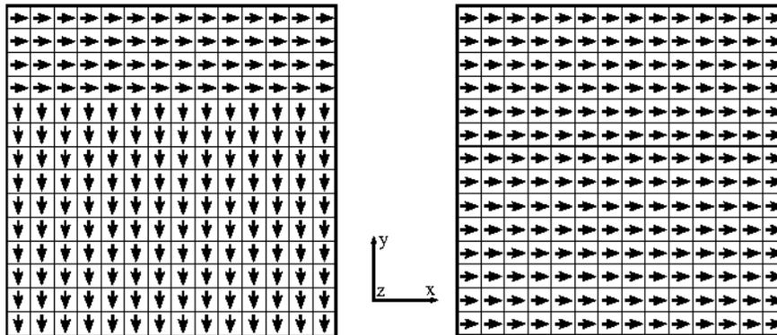
Figure [0-5]. Element directions (N1-N2) of an incoming sheet blank (left) and directions after re-orientation.
