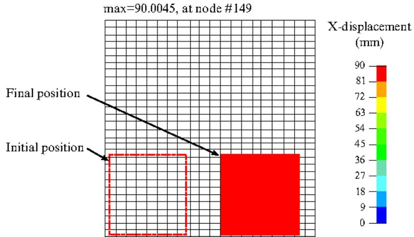
Figure [0-2]. Initial and final position of the blank.
