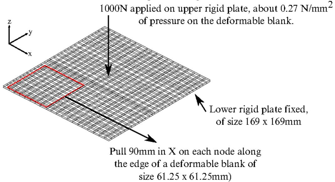
Figure [0-1]. Boundary and loading conditions of a small test model.
