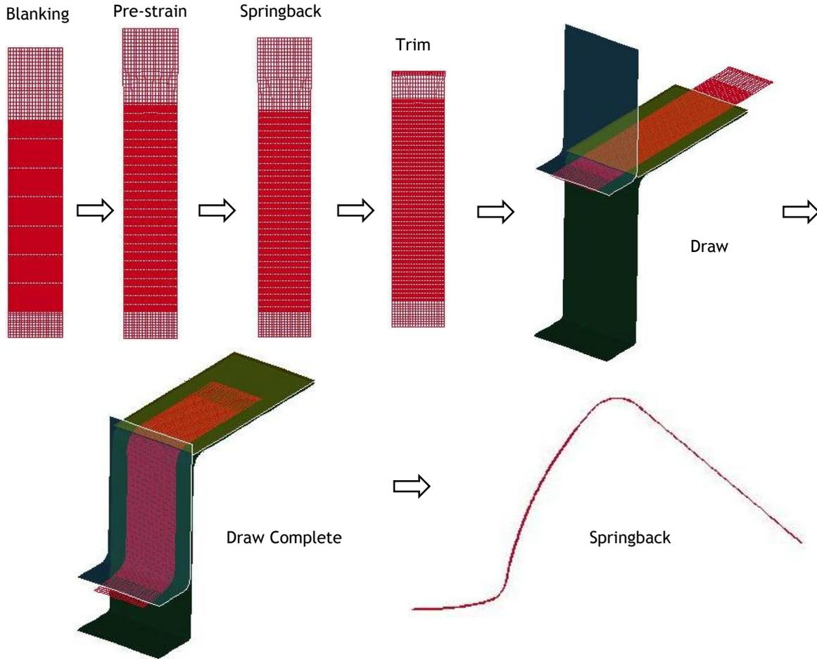
**Figure NUMISHEET2011 Benchmark 4 Simulation process**
