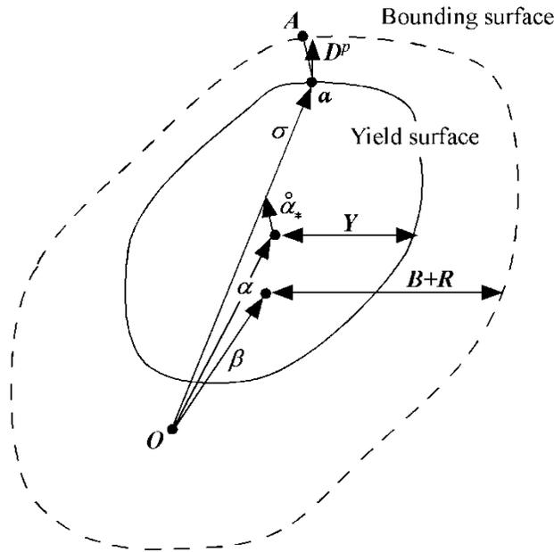
**Figure 125.1** Schematic illustration of the two-surface model
