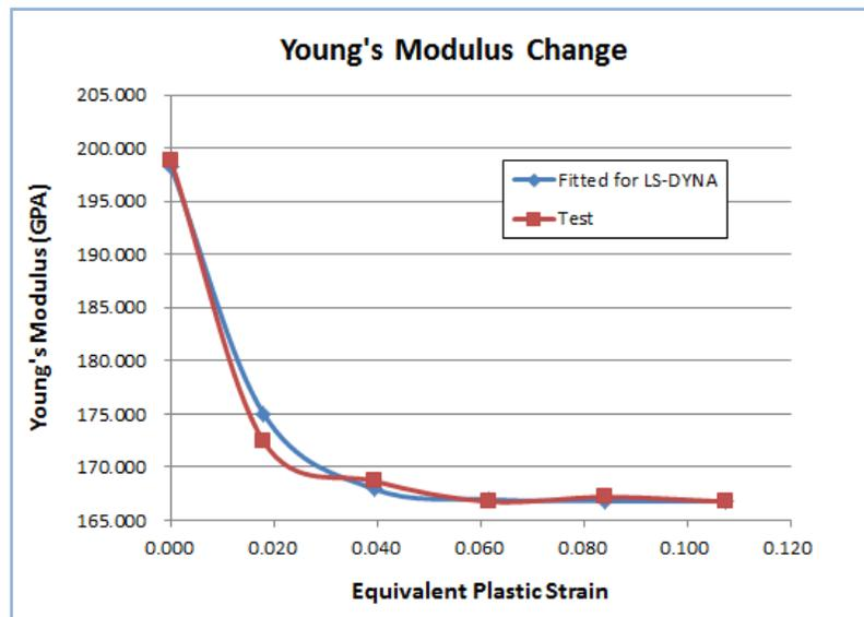
**Figure Curve fitting with coefficients: EA=1.668E+05; COE=95.0**
