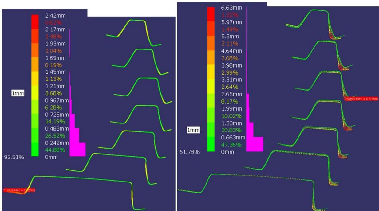
**Figure** Comparison of springback prediction of \*MAT\_125 (left) and \*MAT\_037 (right) on A/S P load beam (*Courtesy of Chrysler LLC and United States Steel*)
