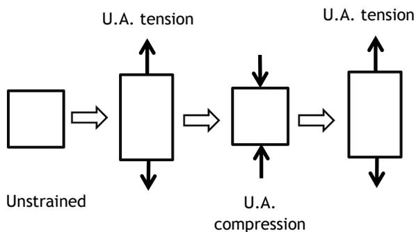
**Figure** Cyclic tension/compression modeling on one shell element
