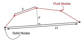
Figure 0-1. Geometry of FSI contact.
