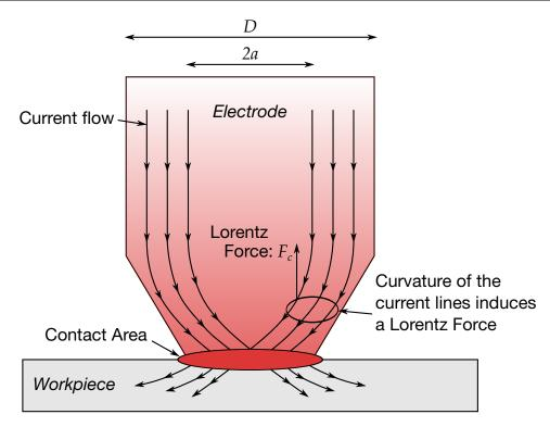
**Figure 6-2.** Electrode coming into contact with workpiece (RSW application).
