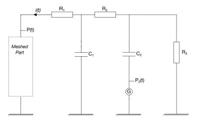
**Figure 7-2.** CV-type circuit
