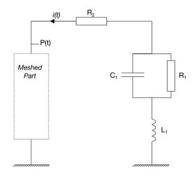
Figure 7-1. Windkessel circuit
