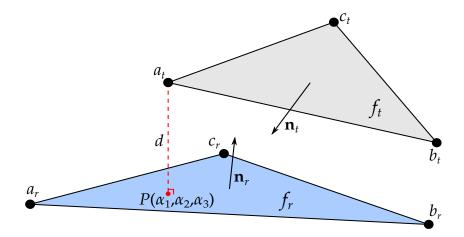
**Figure 0-1.** Contact detection conditions between two faces.
