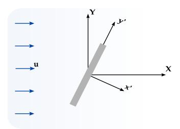
**Figure 7-6.** Anisotropic porous media vectors definition (PMMTYPE = 4, 5, 6, and 7). The vectors  $\mathbf{X}$  and  $\mathbf{Y}$  are the global axes;  $\mathbf{x}'$  and  $\mathbf{y}'$  define the system for the primed coordinate(x', y', z').
